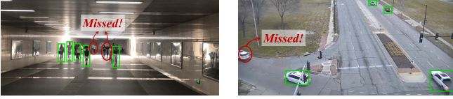
(a) Detect with Low Resolution Fig. 2. Inappropriate Configurations for Detecting Objects
